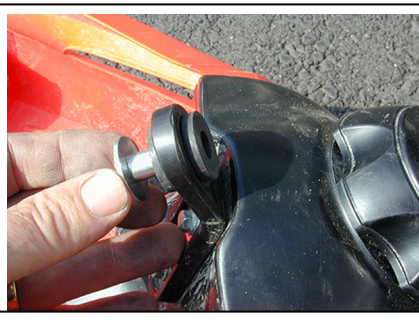
Flip the stock tank bushing over, installed from the bottom. Fender washer goes on the top side.
