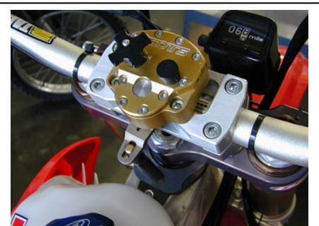
Oversize bars with IMS tank
