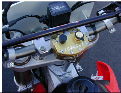
Stock handlebar cross-bar is too close to the damper even in the reversed position mounting.
