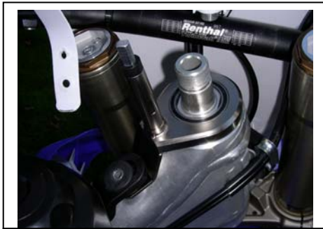
Frame bracket rotates so the tab slides in under the tank bracket mount.
