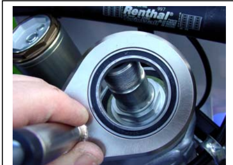
Install the frame bracket and bearing over the new special nut.
