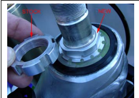
Castle nut off / new nut on / Maintain the same tension on the bearing
