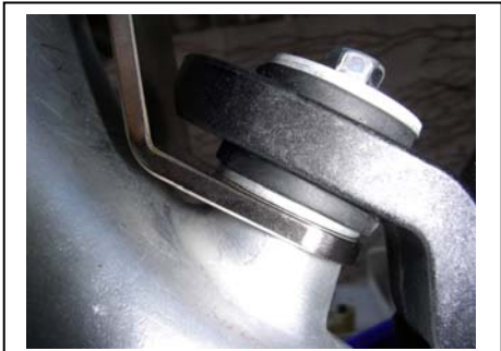
Tab should fit perfectly under tank mount and just slide in over the aluminum frame lug.
