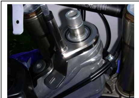
Slide the frame bracket over the special nut with tank tab off to side.
