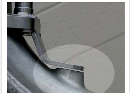
If the frame bracket tab is too low or too high do not try to bend it. Shim it or file the aluminum frame lug a little.
