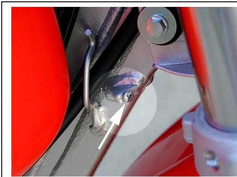
In some cases extending the steering stops may be necessary. Simply insert a screw.>>>
