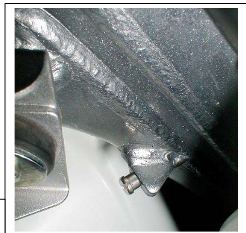
In some cases extending the steering stops may be necessary. Simply insert a screw.>>>
