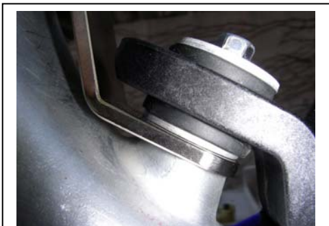
Tab should fit perfectly under tank
