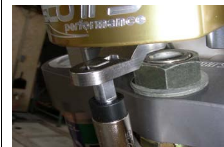
Picture above shows the finished kit. Left: Shows the correct tower pin height when finished, adjusted so the tower pin should be flush with top of link-arm. The black collar can be easily moved up or down on the tower pin to achieve this setting.
