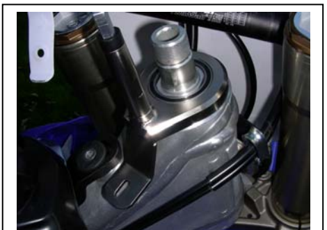
Slide the frame bracket over the special nut with tank tab off to side.
