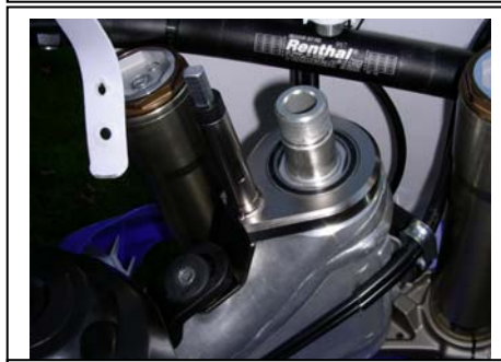
Frame bracket rotates so the tab slides in under the tank bracket mount.
