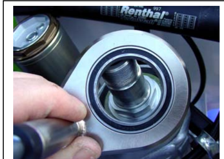
Install the frame bracket and bearing over the special nut.
