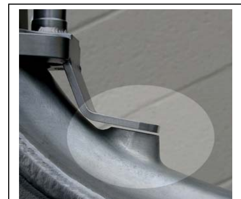
Shim in this case. If our frame bracket tab is too low, file the aluminum frame lug a little, until the tab just slides in. Most bikes fit without mods.
