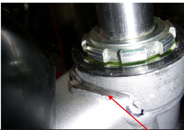
You may need to file the weld downward, here
