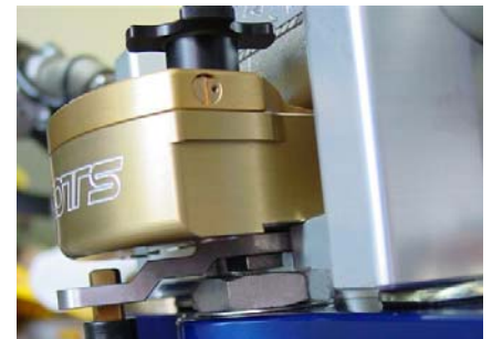
Correctly adjusted tower pin height
