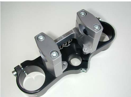
Sub mount on BRP Triple clamps
