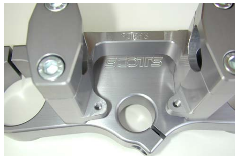
Sub mount on Scotts Triple Clamps
