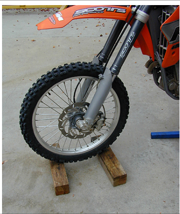
Block the front wheel & forks
