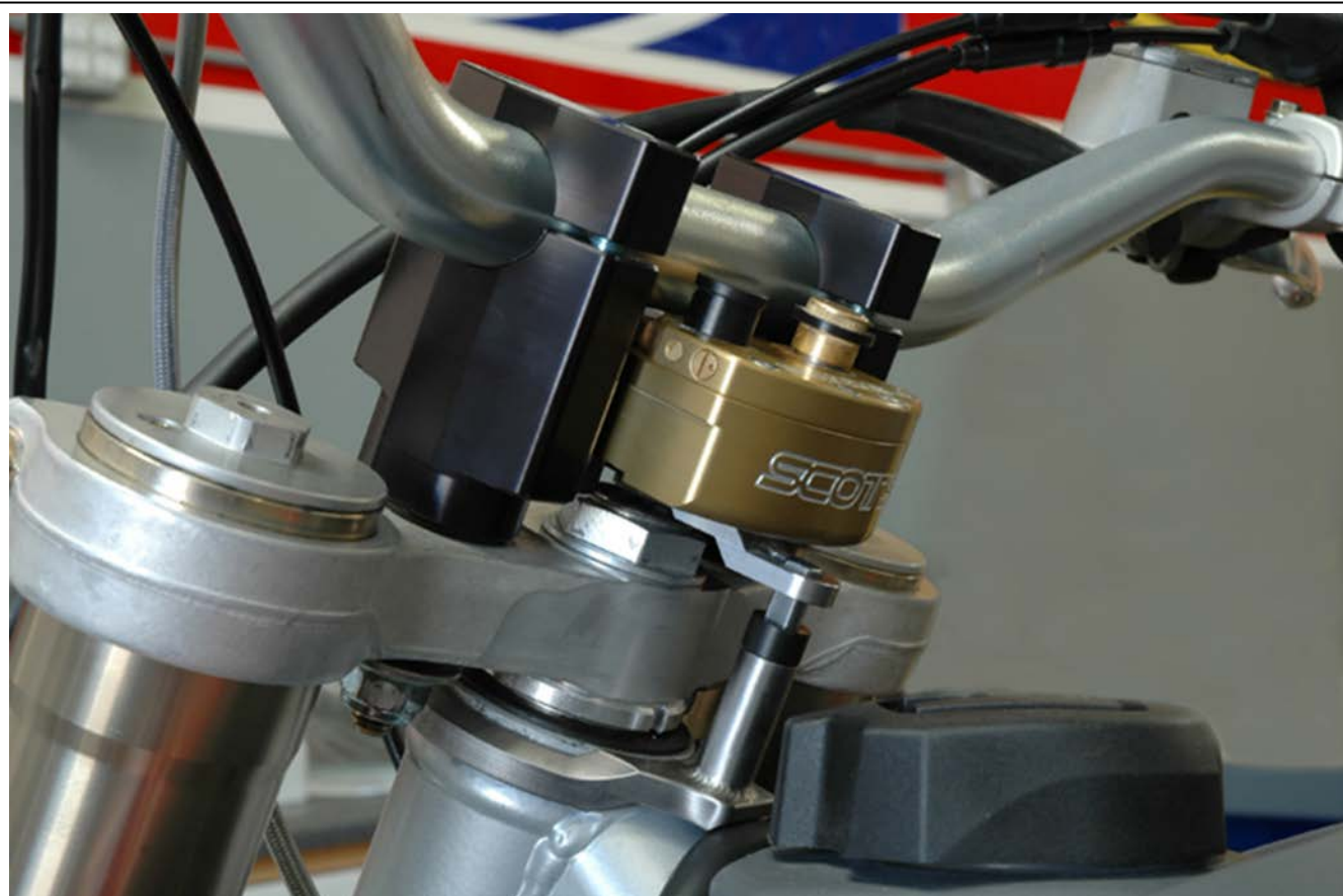
This shows the Sub mount kit complete, mounted on the TE. This is a TE sub mount, the TC looks slightly different.
