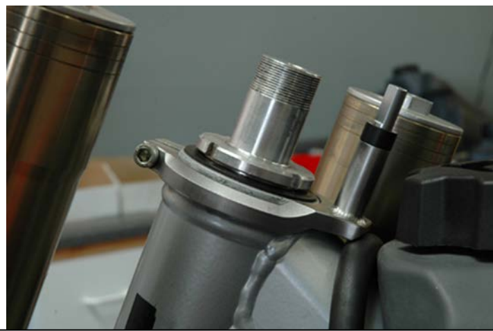
Here is the frame bracket installed, not pinching the radiator hoses and allowing the bracket to clear the nuts on triple clamp.
