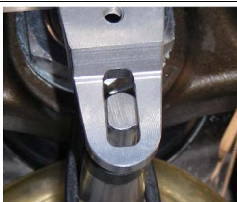
Try to center the pin in the linkarm slot, use welding rod on each side to hold in place.
