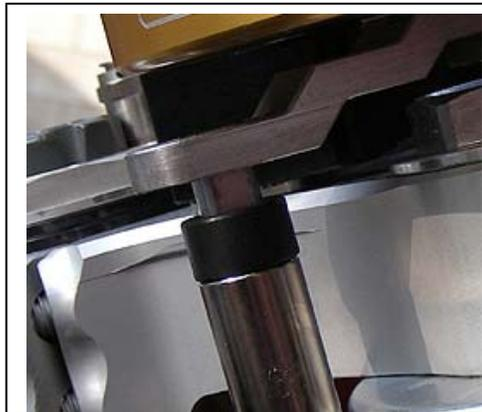
Tower Pin flush as shown, or above top of linkarm by 2mm with rubber mounts.
