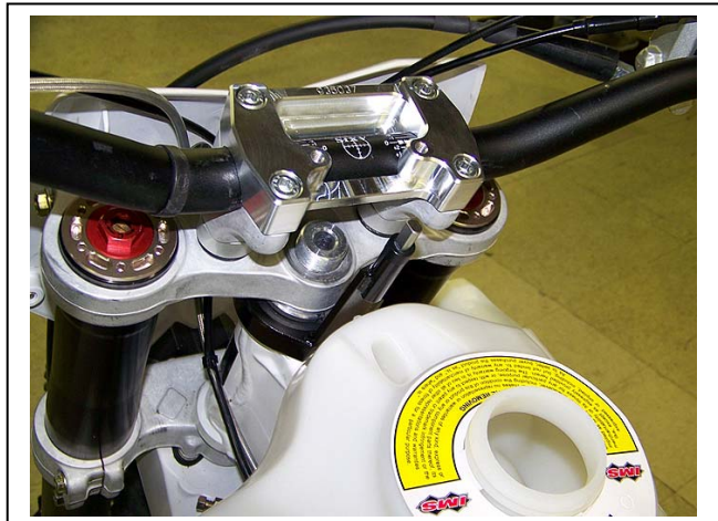
Frame bracket and barclamp installed.
