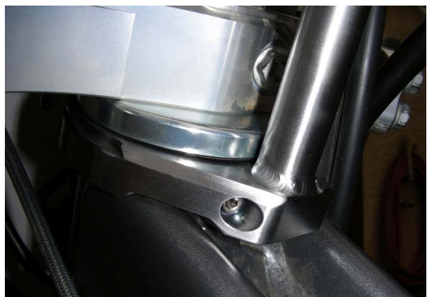
Use BLUE loc-tite (not red) on the set screws.
