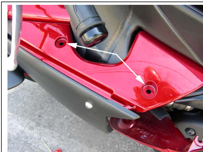
Remove these 2 bolts to gain access to the panel below which allows access to the sheath covering the white plug
