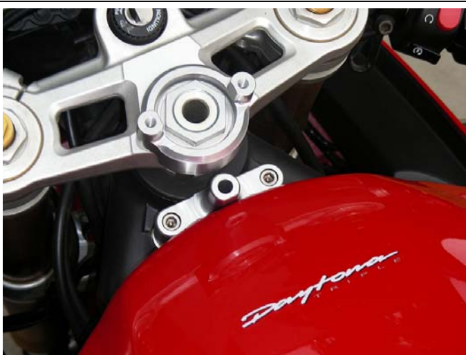
Mounting kit installed properly with 32mm main nut
