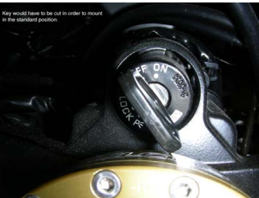
Shows the typical key clearance problem
