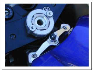
This shows the mounting kit installed before the stabilizer goes on.
