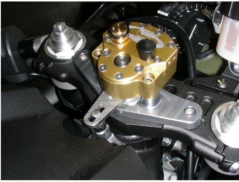
This photo shows the Triple clamp mount (TCM) aligned over the clip-on bolt holes
