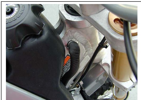
Optional: Re-routing vent tube down the right side.
