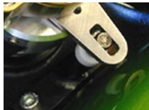
Tower pin location / not binding in slot
