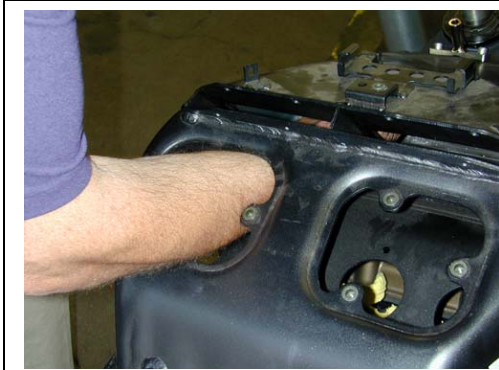
Access to inside of frame for retaining nuts
