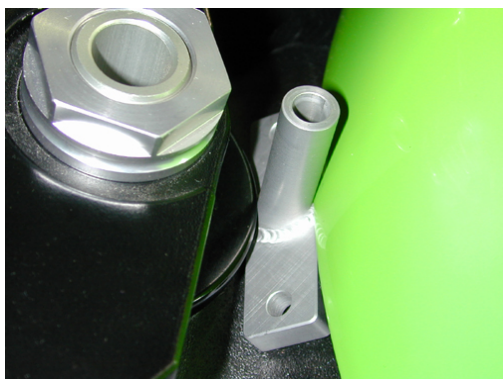
Mark around the bracket & holes, once in place
