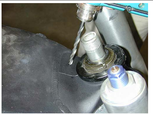
Drilling with triple clamp out of the way
