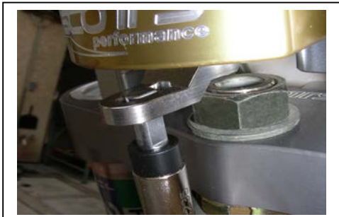
Above: Shows the correct tower pin height when finished, tower pin should be flush.
