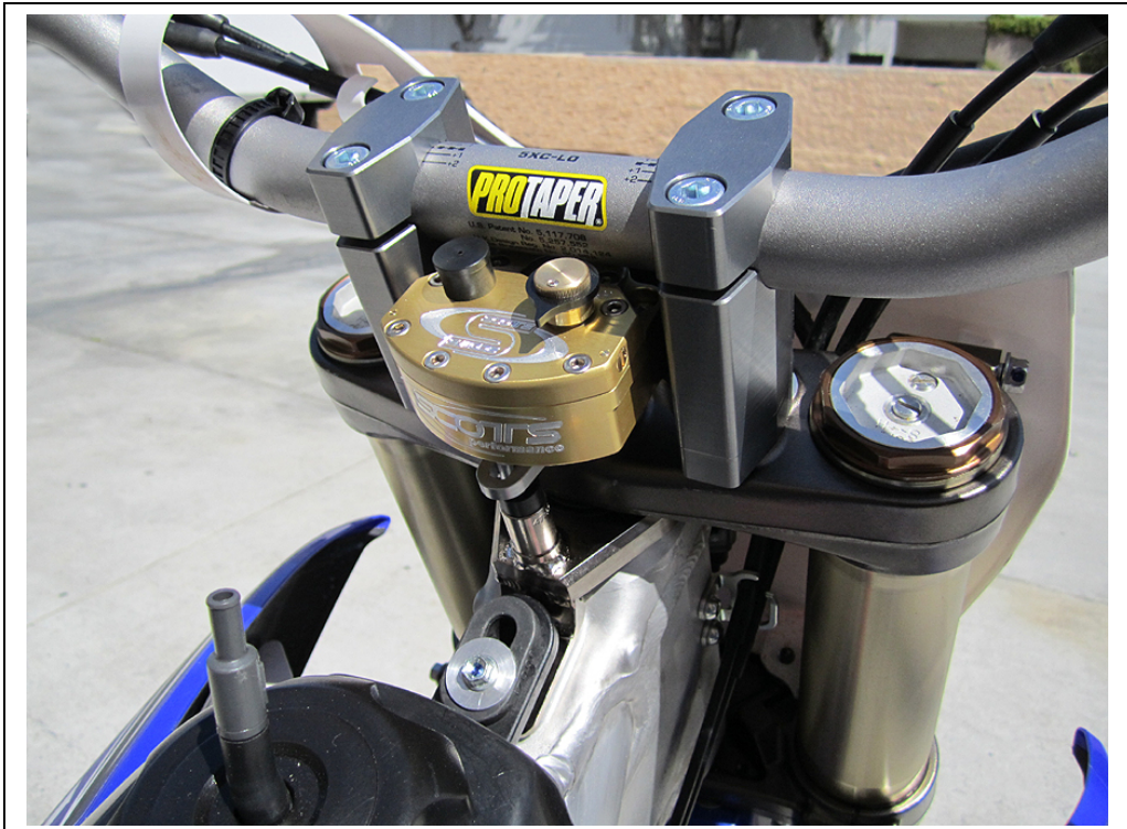
Slide the frame bracket over the special nut with tank tab off to side.
