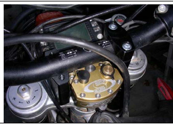
Clutch cable routing is shown here be sure it does not bind at full steering lock.
