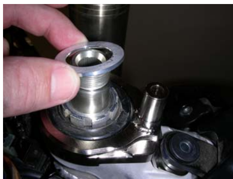
Installing the stem spacer BEFORE the triple clamp is re-installed. This raises the triple clamp allowing clearance between the frame bracket and handlebar bolts.
