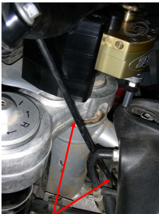
08-09 starter cable routing on outside of sub mount and on rider side of crossover hose.
