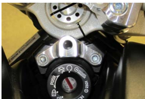
Bolt the frame bracket to the stock key
