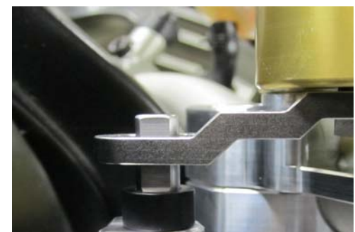
This shows the correct tower pin height
