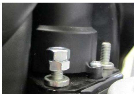
Double nut the key studs to be removed
