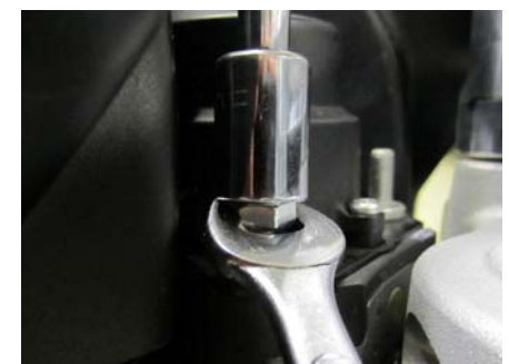
Remove the studs using 2 wrenches
