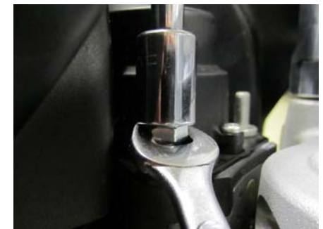
Remove the studs using 2 wrenches
