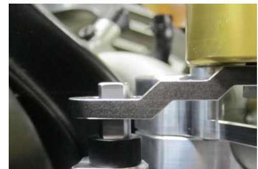
This shows the correct tower pin height
