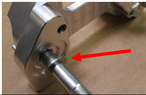
Be sure the stock washers go into the recess area on the bottom of new mount
