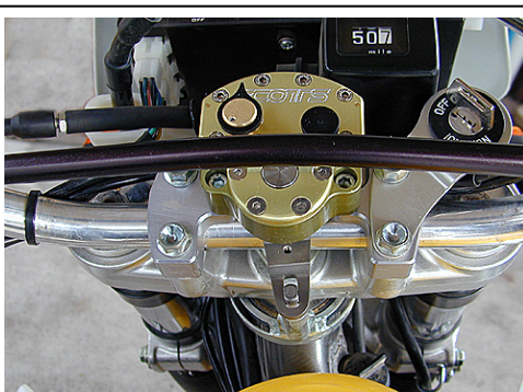
Conventional mount with standard diameter bars, shows "bowed" crossbar.
