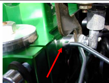
Shows spacer for "S" models between Speedometer mount and triple clamp.
