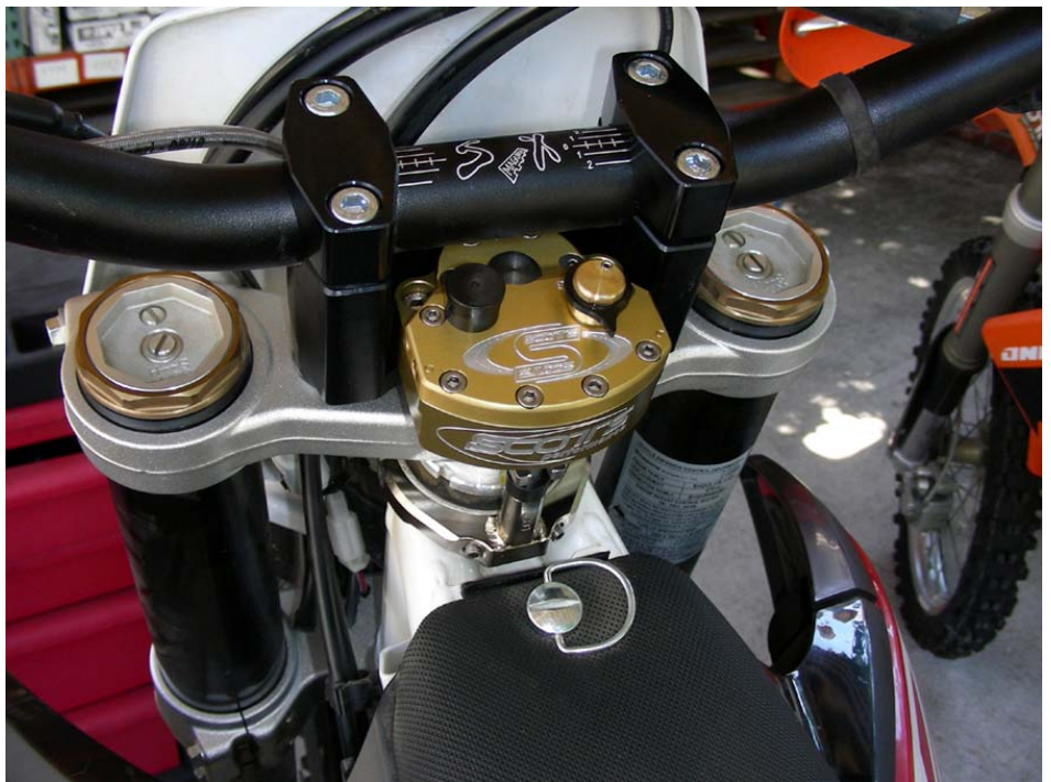
Shown here is the 449/511 Sub mount with Scotts/BRP triple clamp assembly.
