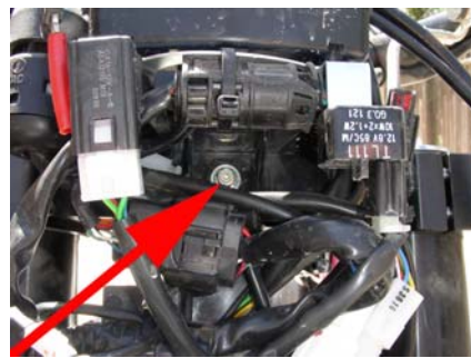
Remove this bolt next which holds the instruments to the triple clamp.
