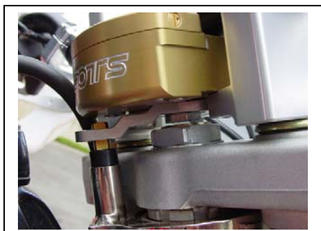
Shows correct tower pin height
