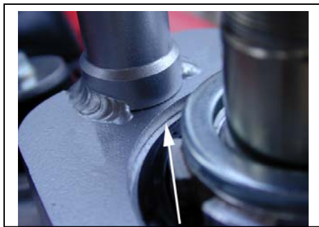
Be sure the frame bracket is all the way down flush with the head tube, all the way around the entire surface.
