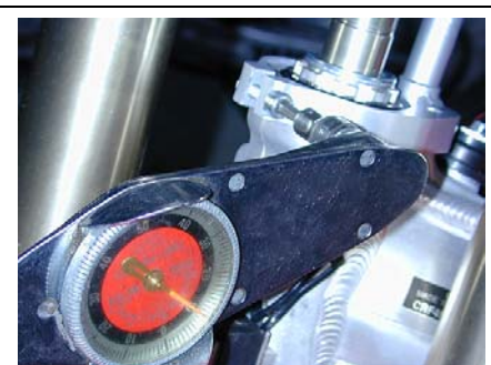
Torque the frame bracket pinch bolt to at least 96-108 inch lbs., or the equivalent of 8-9 foot lbs.
