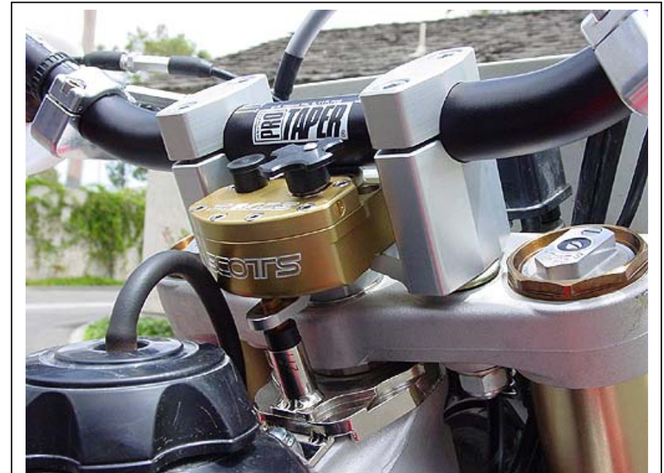
Torque the frame bracket pinch bolt to at least 96-108 inch lbs., or the equivalent of 8-9 foot lbs.
