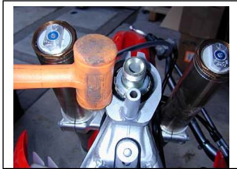
Tap bracket down until securely flush
