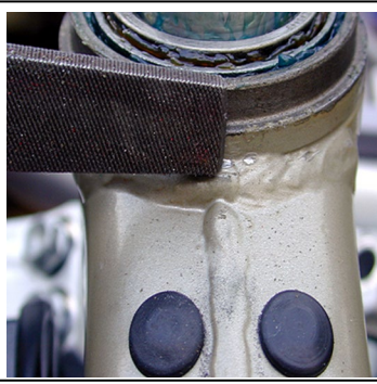
File the high spots and trial fit the bracket until it fits flush.
