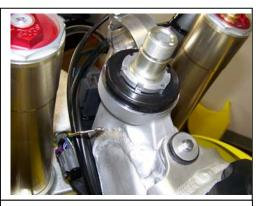
You're going to remove the black dust cover in this picture so the frame bracket can slip over the head tube.
