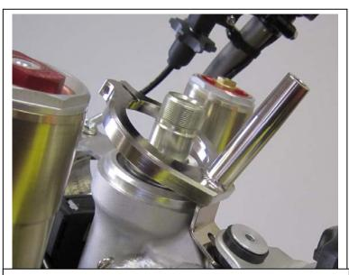
Slide the tab under the tank mount first and then rotate it downward until the ring portion aligns with the head tube. Spread the bracket gently with a screwdriver and let it drop onto the head tube.
