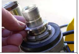
Insert the stem spacer over the stem on top of the jam nut and under the triple clamp.
