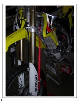
Be sure to tie the forks to the frame as it's very easy for them to roll away from the bike once the jam nut is released on the stem.
