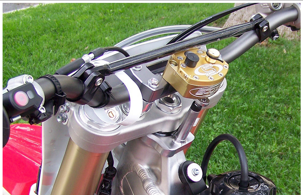
Finished kit installed using the stock handlebars with the stabilizer in the "reversed" position
