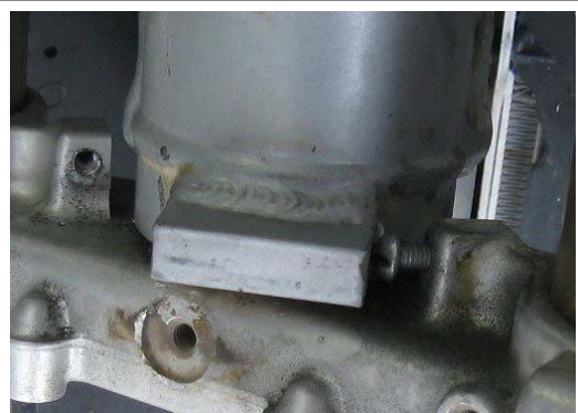
Some models will need to have 5mm bolts installed to limit the steering stops by drilling and tapping the lower triple clamp steer stops and adjusting the bolt so the damper does not serve as the stop. The picture at left gives you the idea of how to accomplish that goal. Allen heads with jam nuts are best, but any 5mm bolt will work. Check these bolts after crashes to be sure they are not bent. If the damper becomes the steering stop then the “shear pin” on the bottom will more than likely do its job and shear off to protect the main vane in the stabilizer.
