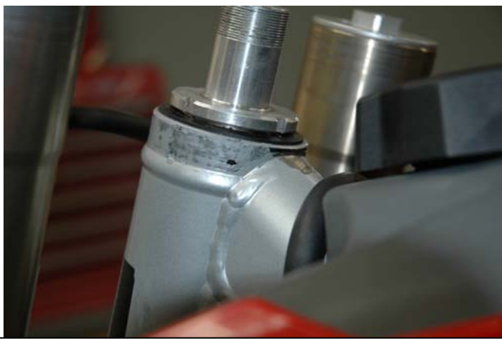
Shown here is some filing at the back of the head tube until the frame bracket is allowed to sit down far enough to clear nuts.
