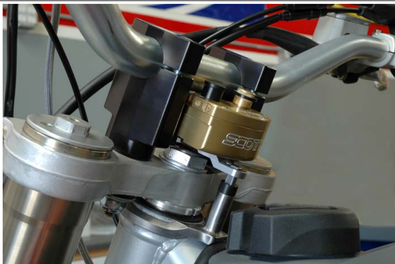
The Black Sub mount in this photo is only to help pronounce the part for the photo and installation ease. The actual Scotts Sub Mount is Titanium in color. Pictured is the TE sub mount.
