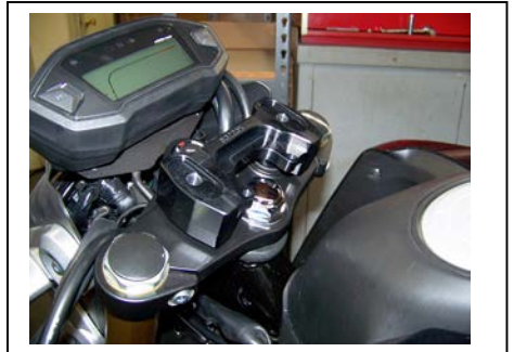
This shows the sub assembly in black installed on the triple clamp
