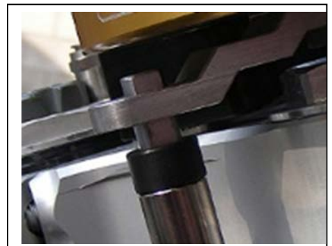
Correct tower pin height
