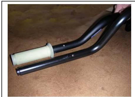
Drill the bars 3/16" to retain controls
