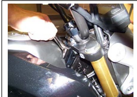
With the 4 tower bolts slightly loosened, slide the assembly into place and install the "through bolts".
