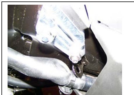
Wire loom routed below bracket
