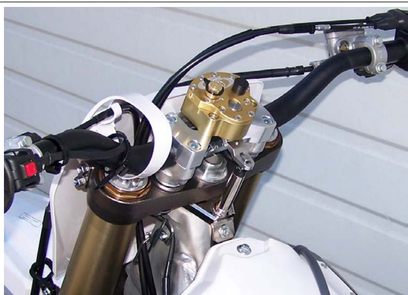
Slide the frame bracket over the special nut with airbox tab aligned. Do not tighten yet.
