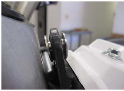
Remove the stock Airbox bushing and install both new bushings.
