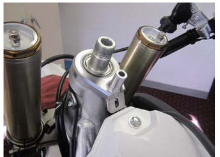
Slide the frame bracket over the special nut with tank tab aligned.
