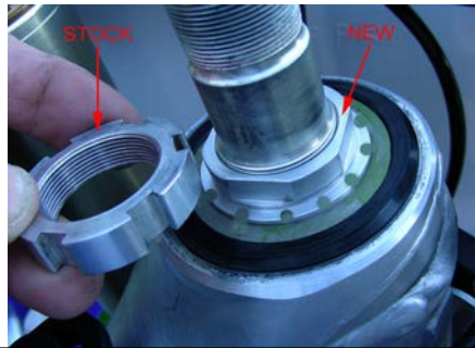
Castle nut removed / new nut installed
