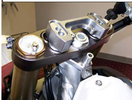
Install the triple clamp with lower sub mount assembly in place, tighten main nut and fork pinch bolts to factory specs. Now you can tighten the tank bolt.
