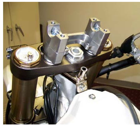
Install the lower half of the bar mounts in the position that suits your riding position, either position #2 or #3. Production Parts are black anodized.
