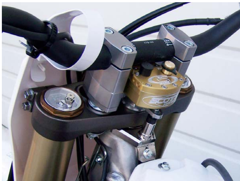
Install the triple clamp with lower sub mount assembly in place, tighten main nut and fork pinch bolts to factory specs. Now you can tighten the tank bolt.
