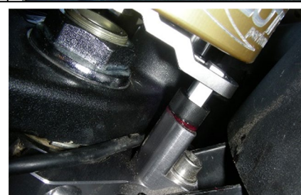
Tower pin greased & installed correctly
