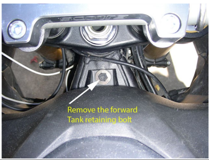
Remove the forward tank bolt
