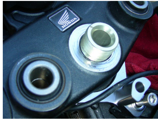
Remove the 30mm nut holding your triple clamp tight to the steering tube
