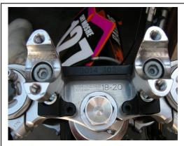
Note how the damper mounting holes are over the center line of the steering stem.
