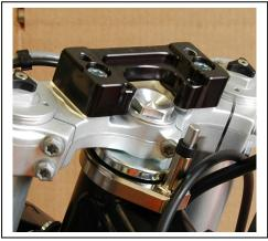
Bolt the SUB mount to the triple clamp, Using the Allen bolts provided.
