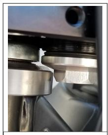
This picture shows the point of the hex on the lower bolt at its closest point. Rotate it so the flat of the bolt head gives more clearance.
