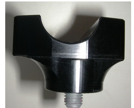
Front of bike is at the left in this picture. This shows the lower Barclamp in the Forward position, centerline of bars are in front of the centerline of bolt.
