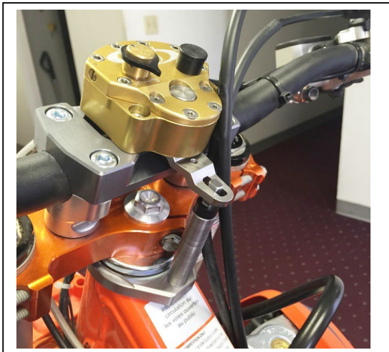
Shown here is the lower Barclamp cradle with the bars in the Forward position. You must tighten the front bolts first, so the Barclamp butts down tightly.
