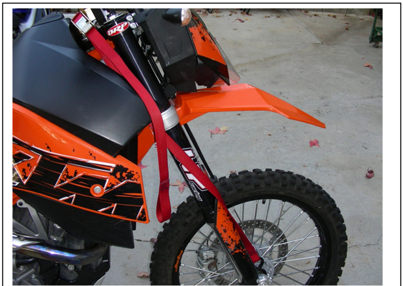
OR: Hook a tie down on the front axle, then up and over the back bone and back down to the other side axle or to the opposite side lower triple clamp to secure the forks in place. This is very important as the forks can roll away from the bike once the triple clamp is off.
