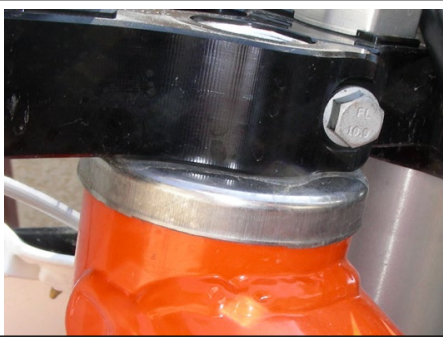
Stock frame welds may need some filing
