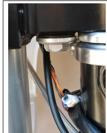
This picture shows the bolt rotated so the flat of the bolt head gives more clearance to the frame bracket pinch bolt area.
