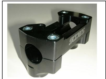
At left shows the new one-piece-Heavy-Duty Scotts lower cradle & Barclamp to replace the rather weak stock unit that bends easily on simple tip overs. A far superior part.
