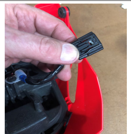
Unplug the headlight by pushing "down" on the tab, not upward.
