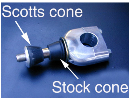
This shows the stock mounting perch assembly but with our cone at bottom.
