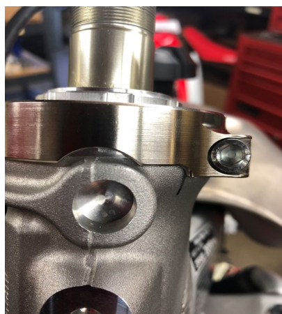
Mount the frame bracket around the head tube and all the way flush.
