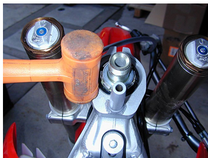
Tap bracket down until securely flush
