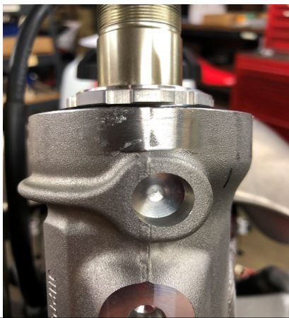
Sand the casting flaws until the frame is smooth and round to mount to.
