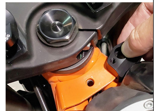
Slide the base plate onto the frame matching up the 8mm hole
