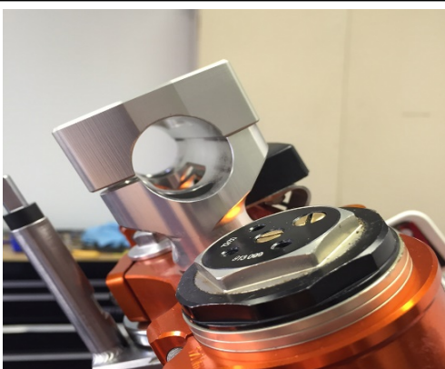
Shown here is the lower Barclamp cradle with the bars in the Forward position. You must tighten the front bolts first, so the Barclamp butts down tightly.
