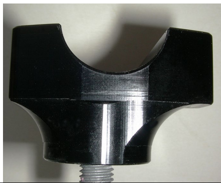
Front of bike is at the left in this picture. This shows the lower Barclamp in the rearward position, centerline of bars are behind the centerline of bolt.
