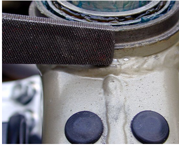
Using a sharp file, start at the high spots and trial fit the bracket until it fits properly.
