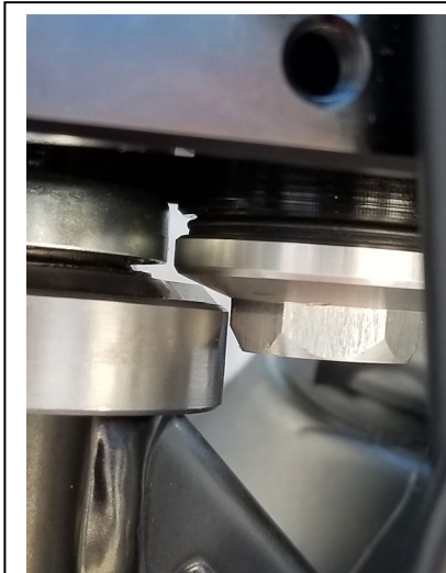
This picture shows the point of the hex on the lower bolt at its closest point. Rotate it so the flat of the bolt head gives more clearance.
