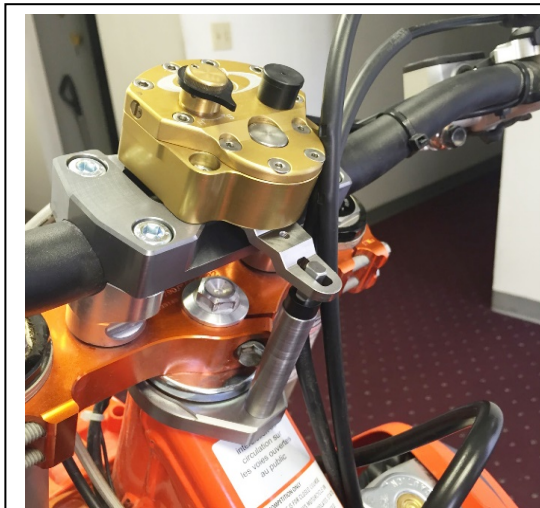
Shown here is the lower Barclamp cradle with the bars in the Forward position. You must tighten the front bolts first, so the Barclamp butts down tightly.
