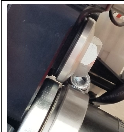
This picture shows the bolt at its closest point to the pinch bolt head, it should be positioned for maximum clearance.
