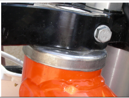
Stock frame welds may need some filing
