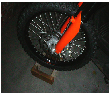
Block the front wheel & forks
