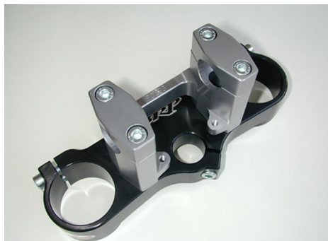
Sub mount on BRP Triple clamps
