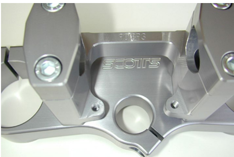
Sub mount on Scotts Triple Clamps
