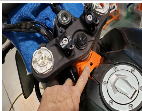
Remove the bars and lay forward in a towel. Remove the frame plug to uncover the 8mm hole.
