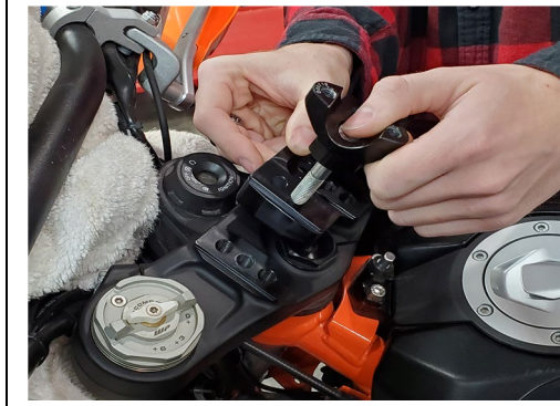
Install the SUB mount base plate to the triple clamp using the desired set of holes
