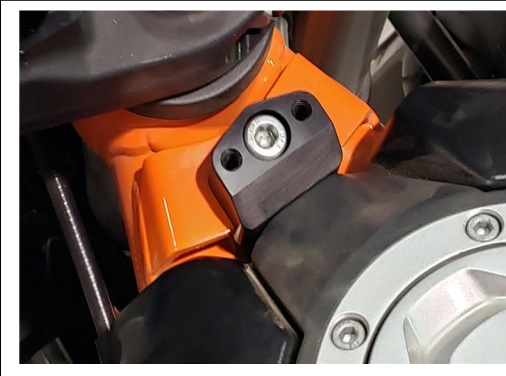
Bolt the lower half of the frame bracket to the 8mm hole in front of the tank
