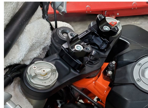
Shows the perches mounted in the Position 3, middle holes, the most common position.
