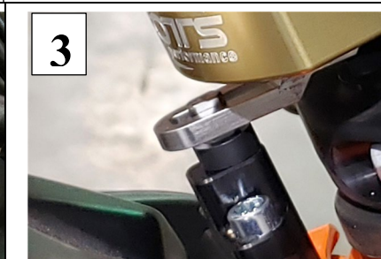
1) Finished kit with link arm and tower pin properly aligned. 2) Lower left shows gas cap open, ready to refuel with key out. 3) Lower center is correct tower pin height installed.
