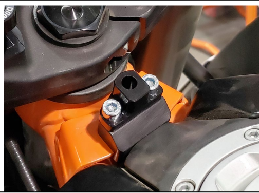
Bolt the upper half of bracket to lower half using 6x20 bolts provided
