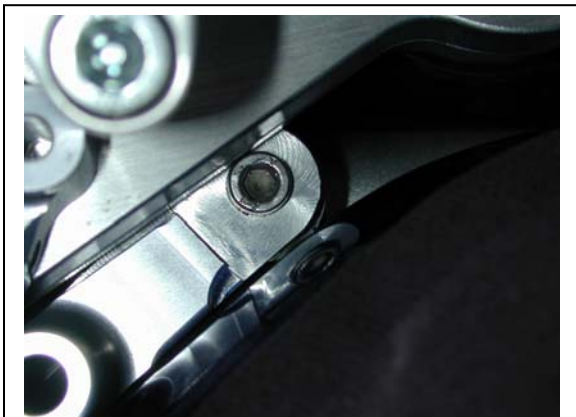
This photo shows the triple clamp at full lock where it actually touches the bolt head of the frame bracket as the steering stop hits too.
