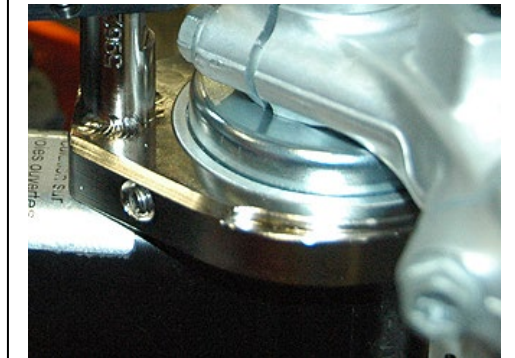
Install the reducer ring, slot to front, and recess facing upward. Flush.
