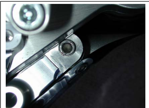
This photo shows the triple clamp at full lock where it actually may touch the bolt head on some bikes simultaneously as the steering stop makes contact.
